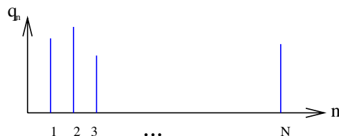
Fig. 1. Like other MC methods, KMC must repeatedly sample from discrete distributions/ensembles. For KMC, this distribution corresponds to a list of rates \{q_n\} that typically changes from one time-step to the next and a corresponding set of events \{\Delta X_n\} that represent local changes to the system state.
